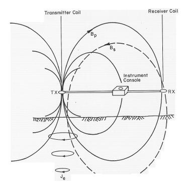
The portable electromagnetic induction unit creates a primary field Bp that induces eddy currents Je In the ground. These in turn produce a secondary magnetic field Bs. The ratio Bs/Bp is indirectly measured by the receiver and is related to the ground conductivity.
